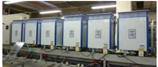
Then, a set of 6 Micronics Systems<sup>®</sup> bipolar rectifiers and computer control software were installed on plating line. Total investment was 47 k€.
