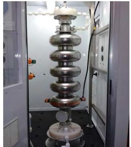
Figure 1: SPL 5 cell niobium cavity. Cavity naming: a) Cell: each one of the elliptical components; b) Cut-off: straight part on top and bottom of the cavity; c) Iris: small section between cells; d) Equator: large section at the middle of each cell.
