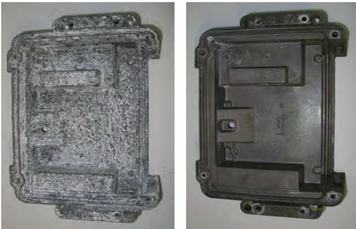
Figure 2: Aluminium cast after 168 h corrosion test EN ISO 9227, left: without passivation, right: treated with the passivation SurTec 650
