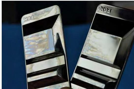
Fig N°9: Aspect of parts treated with STRATA sequence after 480 hours NSST (ISO 9227)
