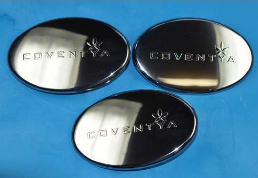
Fig N°8: Aspect of parts plated with STRATA sequence after 96 hours CASS test and PSA thermal cycle
